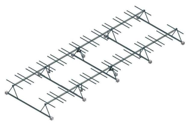
This option consist to join, two by two, the trackers who have their axis aligned from north to south , by a beam-IPN 140.
