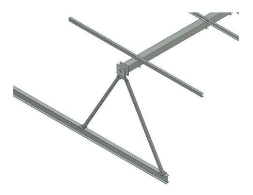
Then make some holes in the ground, in the extreme of each beam, of about 30x30cm and about 20cm deep, and then fills they with concrete to cover also the end of the beam.
