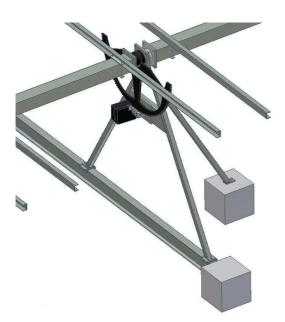
The accuracy mounting the beams and the trackers is not much necesary, but should take care that the maximum angle betwen bars who forms the follower axis should be not more than  $0.7^{\circ}$ . This means that the 6 meters of length of each bar can go up or down (or turn off to the right or left) and vary about 73 mm from the perfect alignment .
