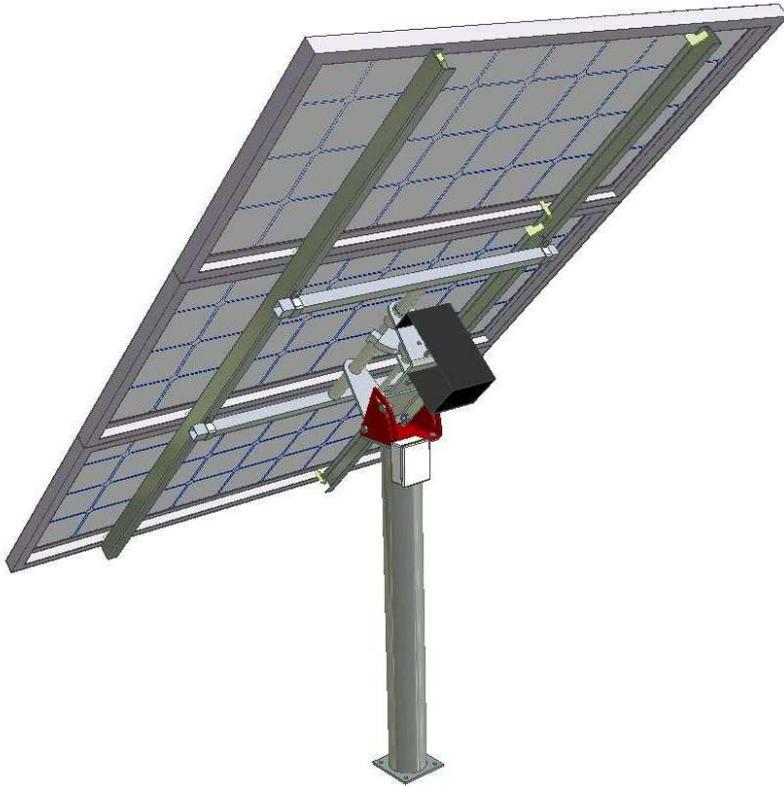
6- The electronic box is put in place, fixing it to one of the screws holding the tracker to the pedestal.
