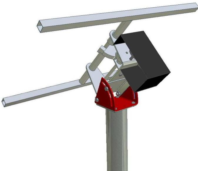
3- The assembly is put in place, fixing it with an inclination corresponding to the latitude of the site. For example, if we are at latitude  $40^\circ$ , we must put it at  $40^\circ$  with respect to the horizontal.
