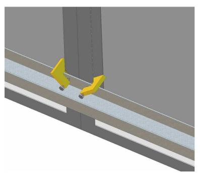
14- Set up the panels with the given bridles as it appears in the illustration.
