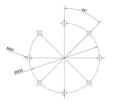
4- A concrete column can be used instead of an iron one. In this case, it should have M20 rods that come out some 60 mm.
