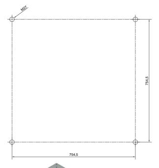
1- Make a concrete foundation , with four M27 threaded rods. They must extend 70 mm out of the concrete. The image shows the distance between the rods.
