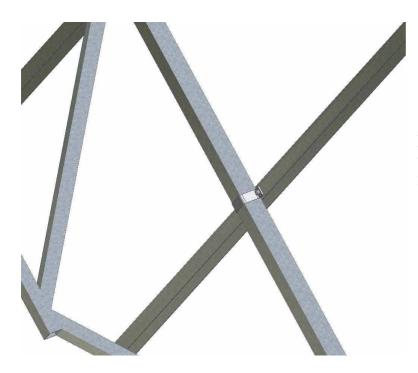
12- We will mount the support bridles of the horizontal bars as shown in the illustration. And we will fix the bars.
