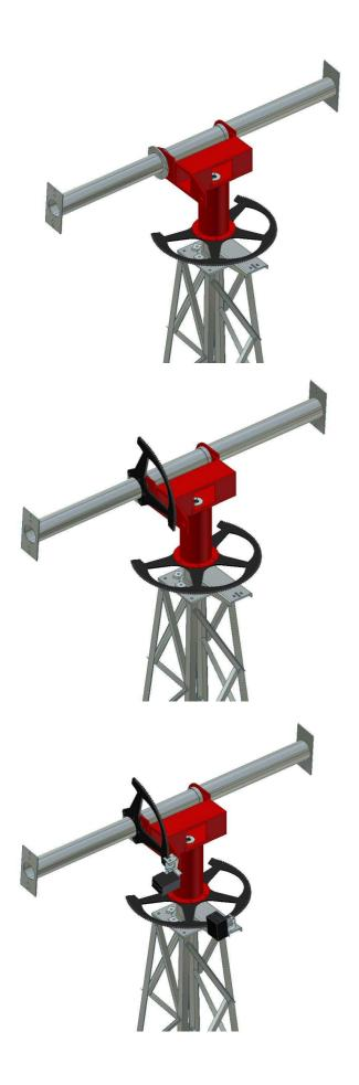
7. Screw on the tube which acts as the main axis in the position shown by the illustration.
