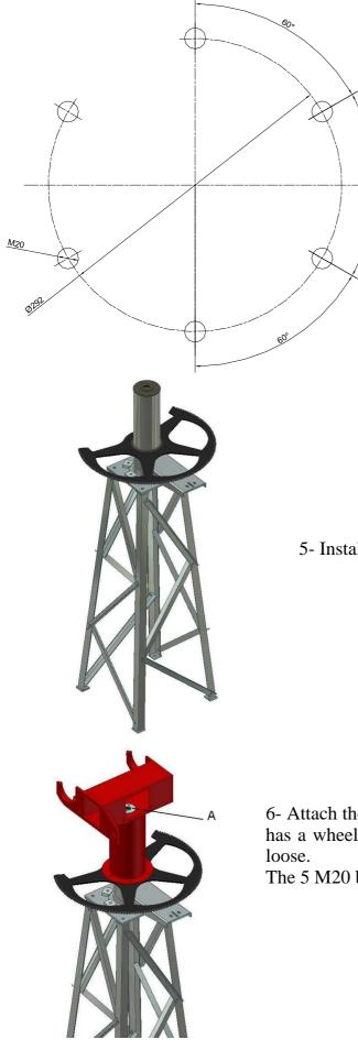
4- A concrete column can be used instead of an iron one. In this case, it should have M20 rods that come out some 60 mm. You can find the measurements in the attached drawing. We can supply a template.
