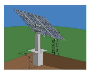
The values are valid for the heights shown in the drawings, for a panel surface of 20 m<sup>2</sup>, for a wind speed of 140 km/h and a safety coefficient of 1.6.
