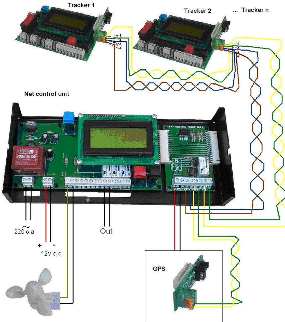
Tracker cable connections, using the RS485 communications protocol.
