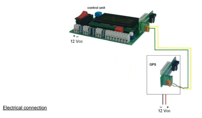
Apart from the connections that are for the tracker's operation, the GPS is connected in a way to show the image. The tracker has a network board that the GPS network is connected to.
